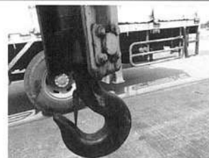
Bottom hook : Normal condition
