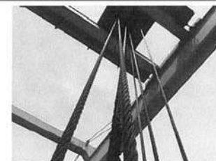
Sheave and wire rope: Normal condition
